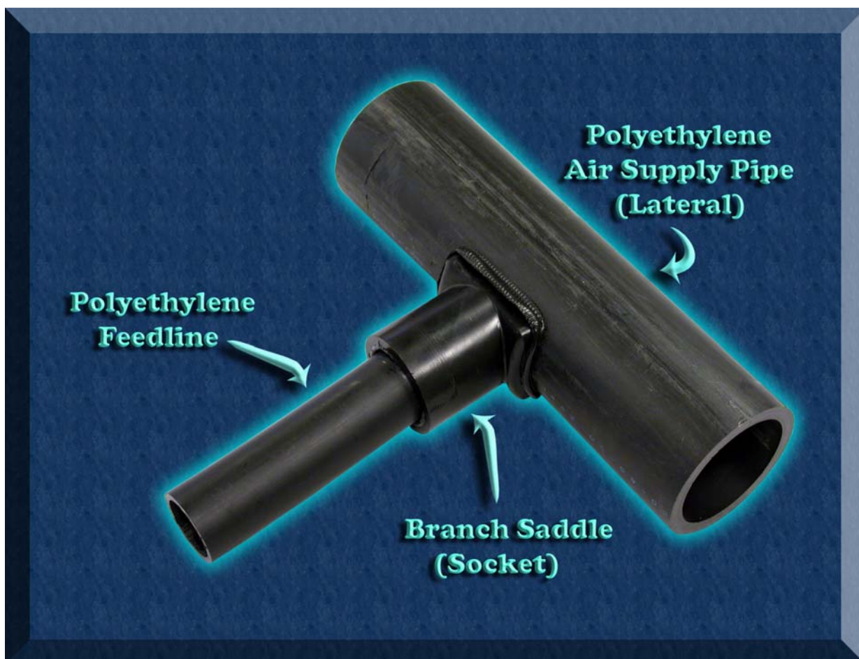
PE feedline socket thermal welded into branch saddle which is saddle thermal welded to lateral pipe.
